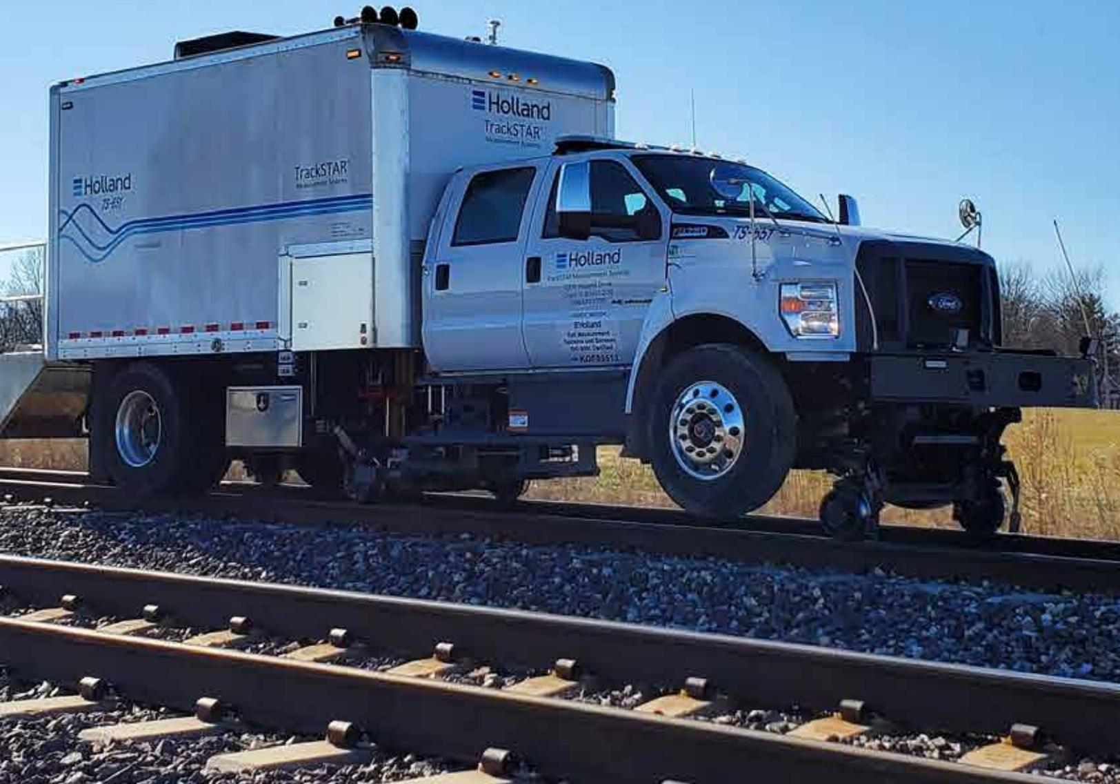
Using Holland's proprietary Argus® track measurement technology, we offer multiple applications to test your track condition.
