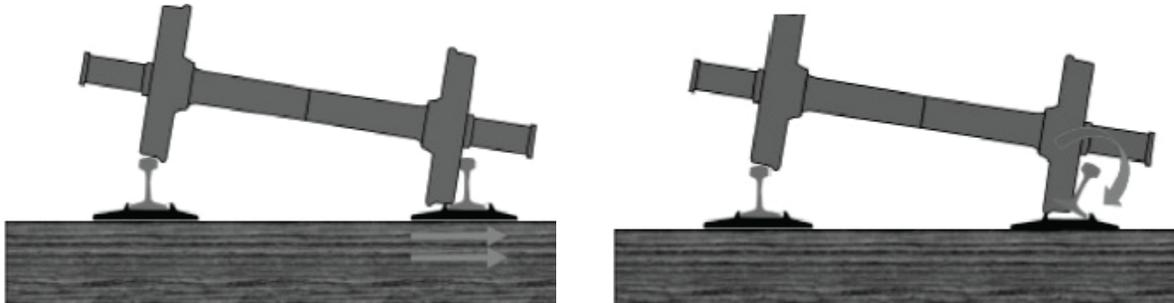
Figure 1 Gauge Widening and Rail Rollover
