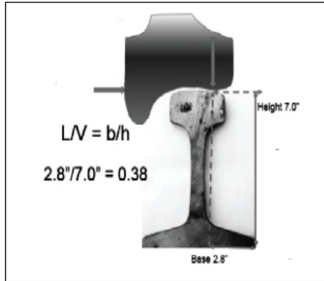
Figure 3 Reduction of B/H Ratio with Hollow Wheel Field-Side Contact - Low Rail
