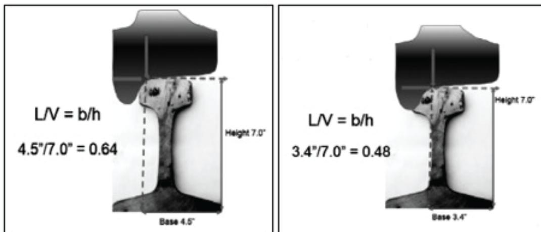
Figure 2 Reduction of B/H Ratio With Gauge Face Wear – High Rail
