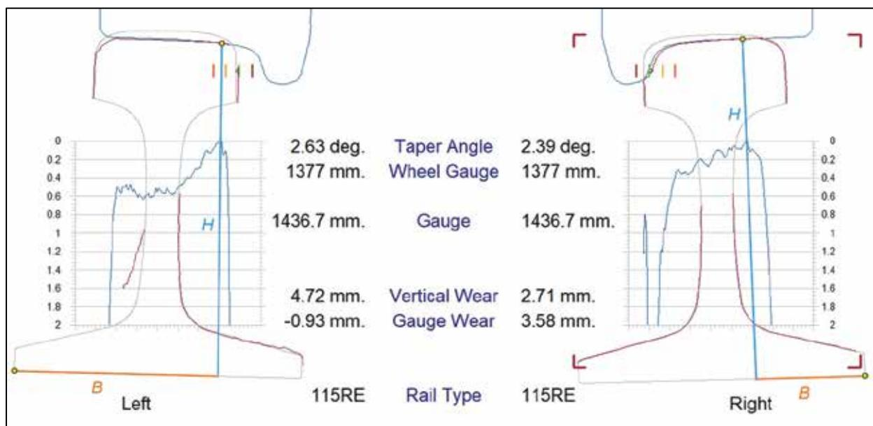
Figure 7 Rangecam B/H Ratio Calculation Example
