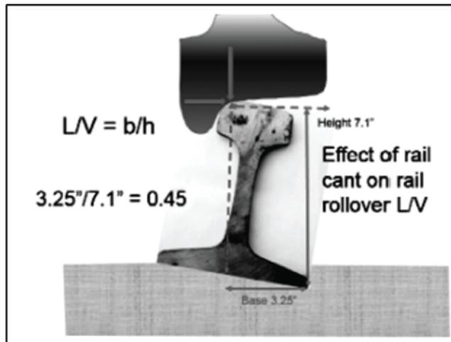
Figure 4 Reduction of B/H Ratio with Reverse Rail Cant
