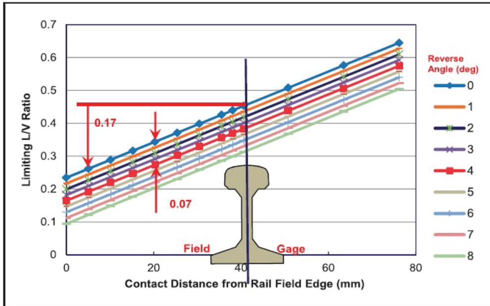
Figure 5 L/V to Initiate Rail Rollover as a Function of Rail Cant Angle and Lateral Contact Position (Wu & Kerchof)
