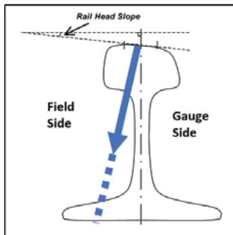
Figure 6 Railhead Slope
