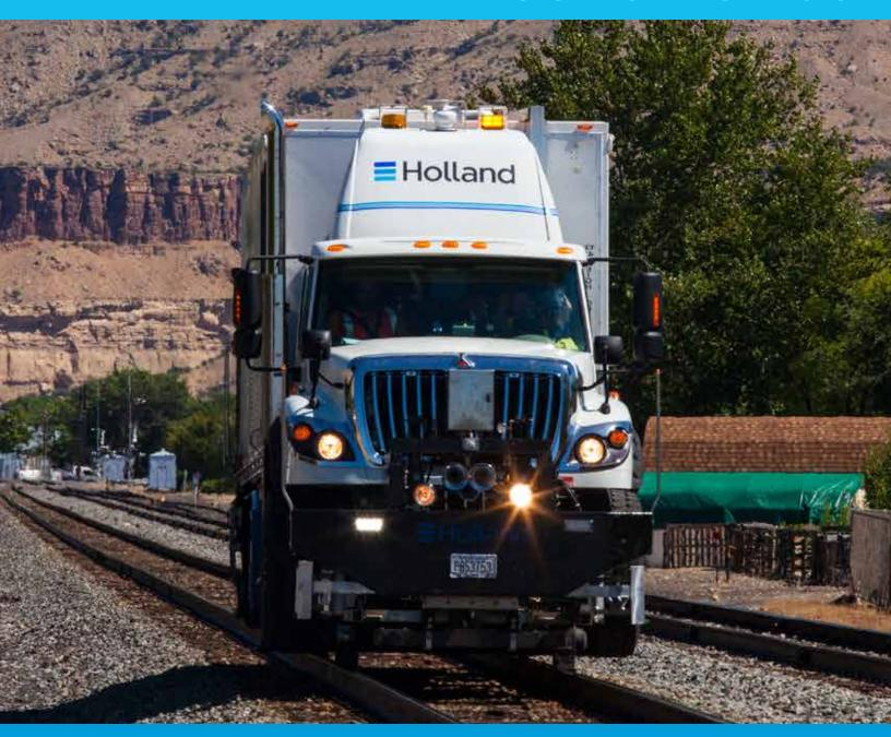
Using Holland's proprietary Argus® track measurement technology, we offer multiple applications to test your track condition.
